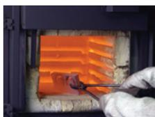
While beryllium-containing alloy heat treating operations do not generate any beryllium-containing fume, spalling of the surface oxide during subsequent material handling steps can cause exposures which must be controlled.
